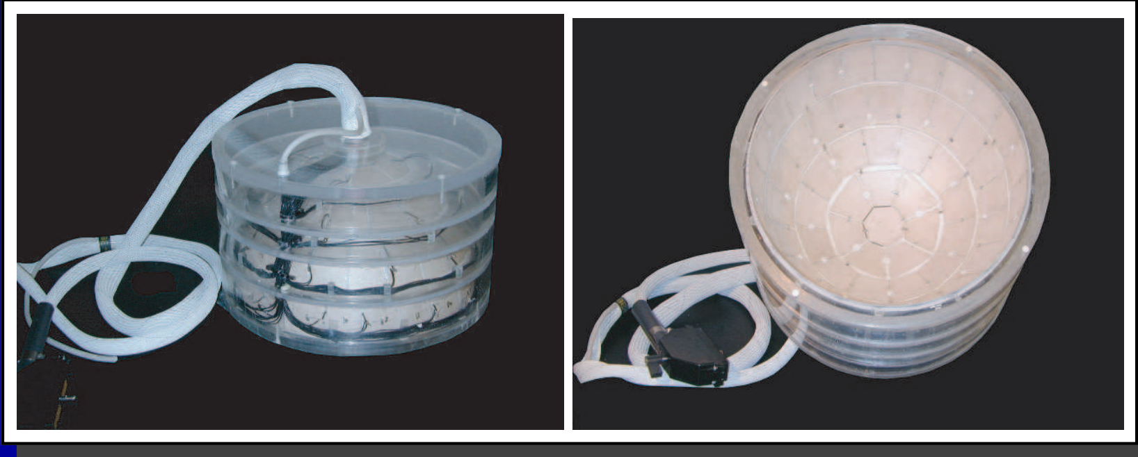
Figure 5: A Phased array for brain surgery.
