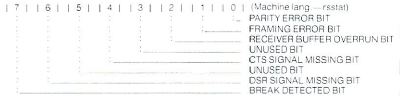
Figure A-3. RS-232 Status Register
